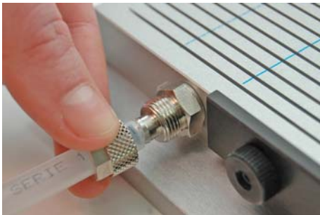
Fig. 3: Connect the vacuum hose
