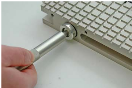
Fig. 5: Remove the blanking plugs
