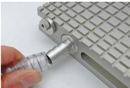
Fig. 3: Connect the vacuum hose
