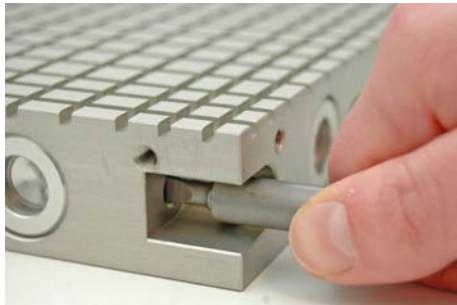
Fig. 4: Release the screws
