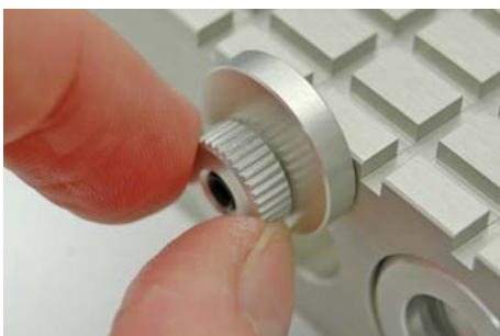
Fig. 9: Tighten the stop washer
