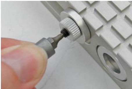
Fig. 8: Install the set screw
