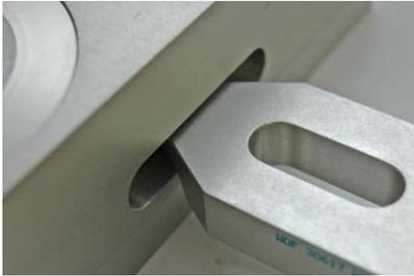
Fig. 3: Attaching the clamping jaws
