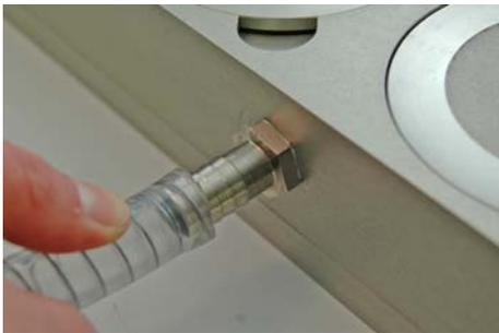
Fig. 4: Connect the vacuum hose
